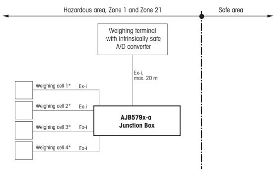
\* Weighing cells must be approved for the hazardous area.
