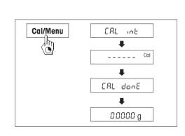
To obtain accurate weighing results, the balance must be adjusted to match the gravitational acceleration at its location.
