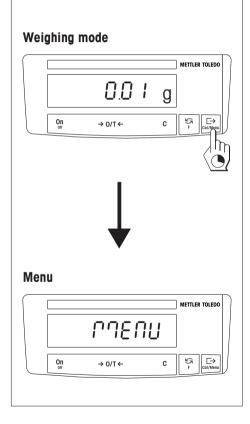
The balances have two operator control levels: the **weighing mode** and the **menu**. The function of each individual key depends on the operator control level and how long the key is pressed.
