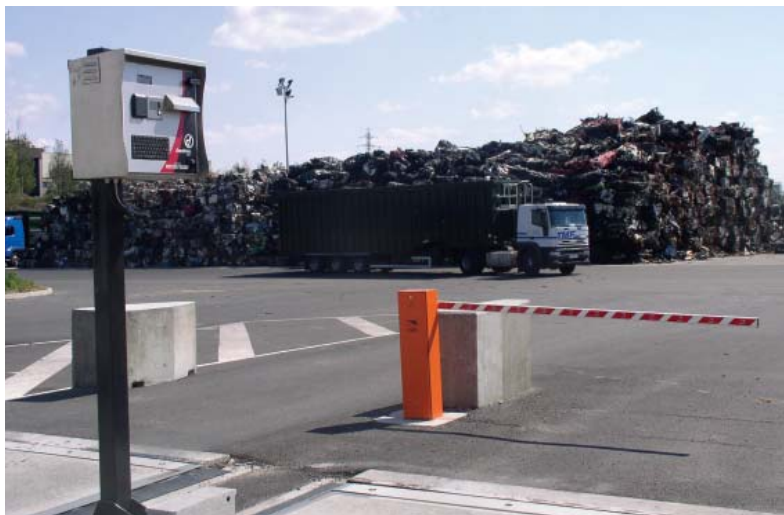
Unattended driver terminals keep traffic moving over scales by allowing drivers to process their own transactions in seconds.
