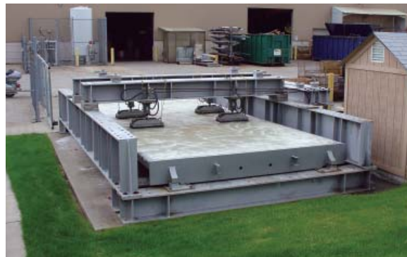
The module masher tests truck scale modules by simulating 20 years of traffic within 2 months.
