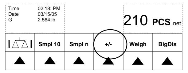
6. When ready to checkweigh the carton, the operator touches the "+/-" softkey. Scale switches to +/- Checkweighing mode.
