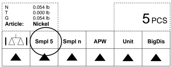
If the operator places the wrong sample quantity, say six pieces, or the wrong parts, say quarters, then the Smart+ will display out of tolerance message.
