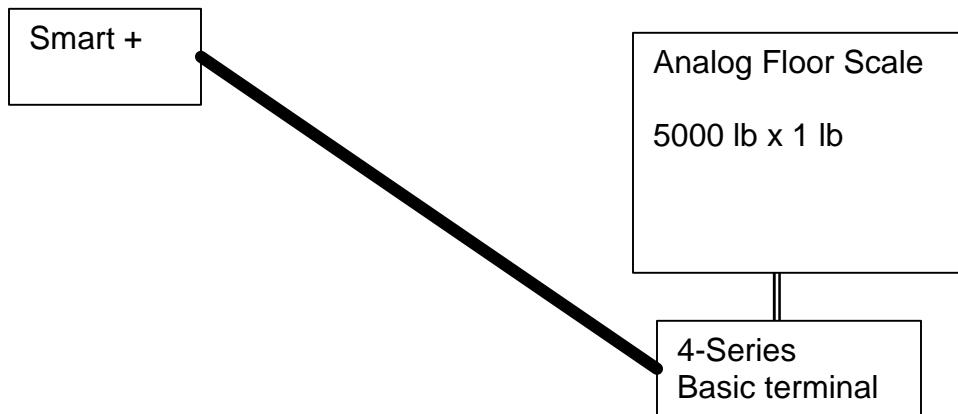
If the average piece weight (APW) of the parts is 0.05 lb and the bulk scale division size is 1 lb, the bulk count will update by 20 pieces; 10,000, 10,020, 10,040 etc.
