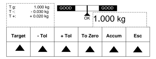
In this demo we show how to send targets with tolerances via a PC over a com port, the COM Port can be RS232, USB or Ethernet.
