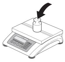
After choosing the calibration weight, place the weight on the weighing pan and then press the **«OK»** softkey.
