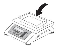
Place the **empty** weighing container or packaging on the scale and then press the  $\leftarrow$ T  $\leftarrow$  » key briefly, or press the  $\leftarrow$ PT » softkey if a **known tare** weight has already been established.
