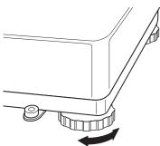
Turn the adjustable feet so that the scale is horizontal. If a spirit level is filled, the bubble must be located within the inner circle.
