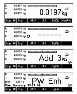
10 samples were placed on the scale and **«Smpl 10»** was pressed.
