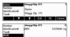
Press **Define** to modify the selected article. Select the desired parameter by using the **A**, **A**, or **B** softkeys, then press **Edit** to modify the selected parameter.
