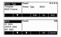
Choose "Printer Type" and press the «**Edit**» softkey to define the printer.
