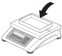
Place the **empty** weighing container or packaging on the scale.
