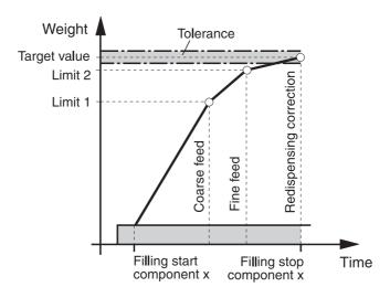
If no limits are entered for an individual component, the ID7-Dos-R automatically determines Limit 1 and Limit 2 in the learn mode, see section 3.1.2. The target weight of the component is then exactly achieved.
