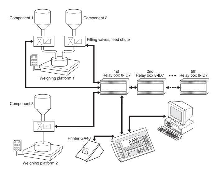
The control signals for the dispensing valves of the individual components are transmitted via the RS485-ID7 interface to up to five 8-ID7 relay boxes. The 8-ID7 relay boxes control the dispensing system either directly or via an additional external control unit (PLC). The components can be picked up directly or with binary coding (see section 7.1).
