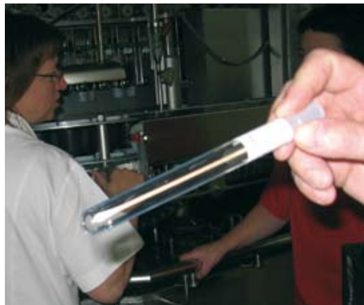
Taking swap samples from the production line into the tube containing culture medium for microbiological control.
