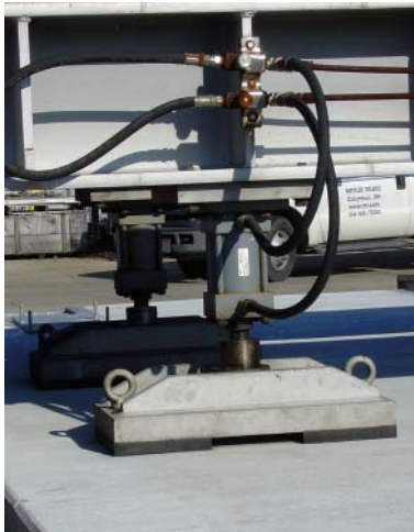
Each foot is equipped with two rubber pads spaced like a pair of tires.
