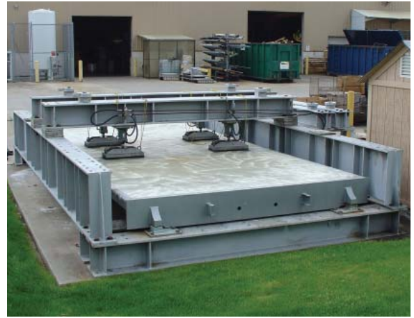
The module masher tests truck scale modules by simulating 20 years of traffic within 2 months.
