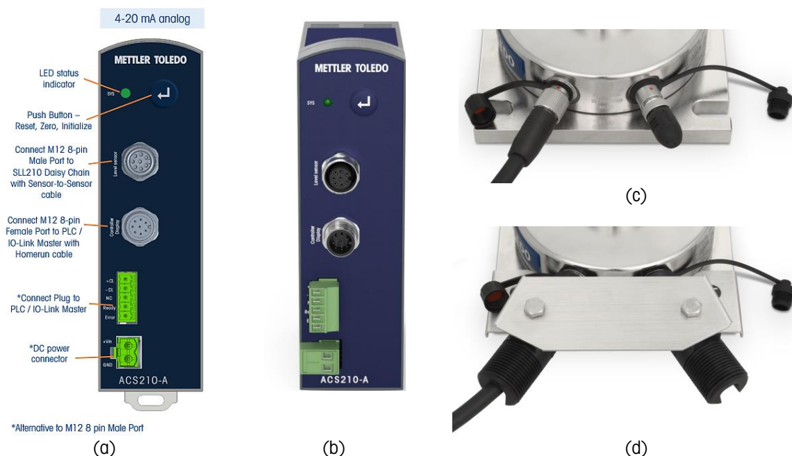
Figure 20: LED Push Button has been integrated to the ACS210 unit to mechanically configure the daisy chain (a,b), the daisy-chain is terminated with the terminal resistor (c,d).
