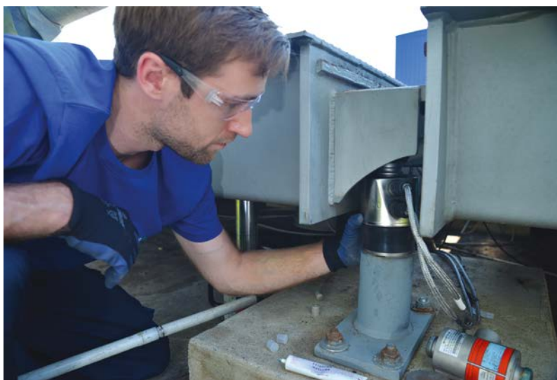
Conversion kits make it easy to upgrade existing vehicle scales to POWERCELL® PDX® load cells.
