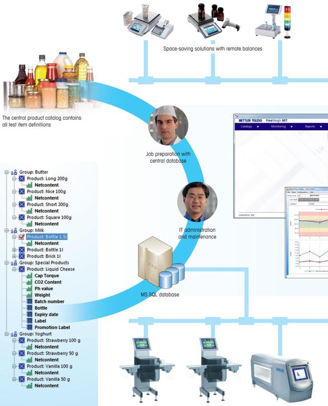
Automated checkweighing and metal detection
