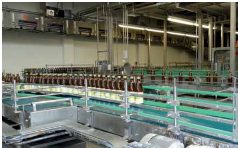
Bottle filling with fill level tolerance of maximum 1.5 percent
