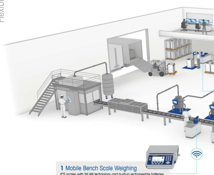
ICS scales with WLAN technology and built-in rechargeable batteries can be placed exactly where they are needed at any time. They also offer convenient data transfer for external data storage or updates.
