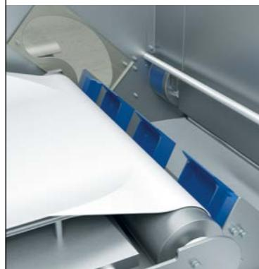
X-ray inspection systems with multi-lane reject devices can reduce waste by rejecting a smaller amount of product instead of rejecting the full belt width. Adjustable positioning of the reject scoop provides complete flexibility to cover a range of application and line speeds.
