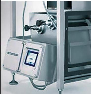
For high-value powders and dusty products, a seal-tight reject mechanism within a gravity fall metal detection system is recommended. The dust-tight seal minimizes the amount of 'good' product that gets rejected, reducing product waste.
