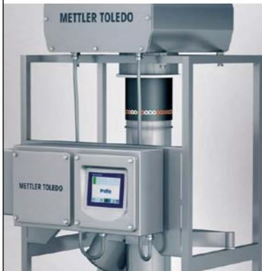
A gravity fall metal detection system is often used when inspecting free-falling powders and fine granular products. High speed, pneumatically controlled y-valve reject devices minimize the amount of good product rejected when metal is detected.
