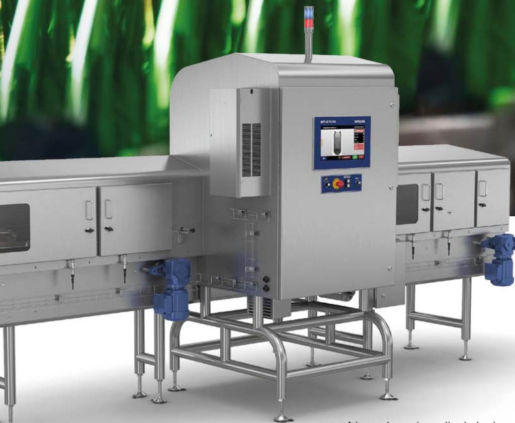
Advanced x-ray inspection technology for glass-in-glass contaminant detection
