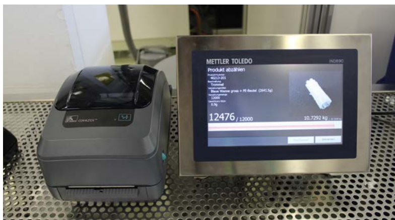
The counting bar graph on the terminal indicates the fill level.
