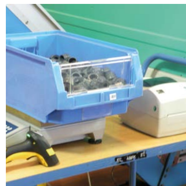
Scales attached to printers supply labels instantly for speedy processes and traceability.
