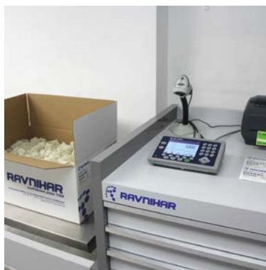
Optimal counting station – platform, terminal, scanner and printer.
