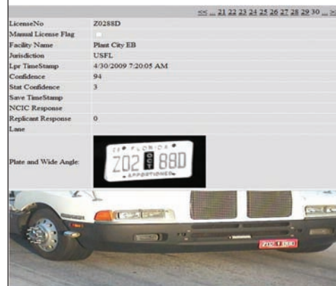
LPR record showing IR images of plate and OCR text.
