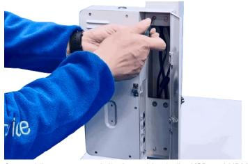
4. Connect the camera and display cables to the USB and HDMI interfaces.
