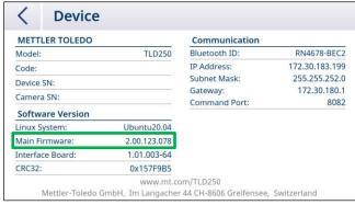
**Note:** If the main board firmware upgrade keeps failing, please consider calling technical service for a new solid-state disk (SSD) memory card.
