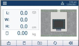
2. Place the object on the base plate or the weighing scale, within the Autosense zone, (blue box - dashed line). Wait until the motion symbol disappears.
