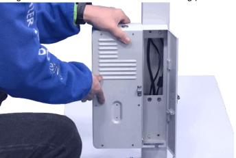
3. Fasten the electronic module with four M4 pan-head screws. Tool: Phillips screwdriver.
