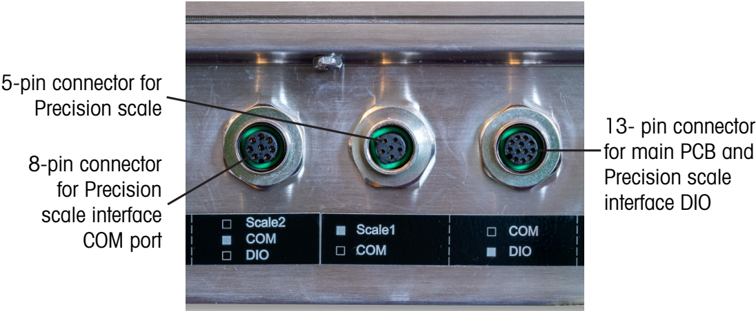
Figure 47: External M12 Connectors Associated with Precision Interface Board
