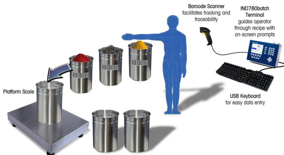
Figure 15-12: IND780batch Manual Formulation System Diagram
