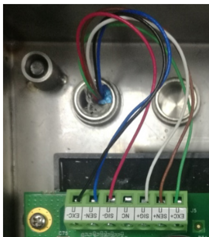
Figure 4-3: Analog Load Cell Connection Terminal
