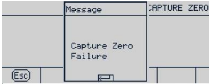
Figure 1-13: Zero Calibration (Failed)
