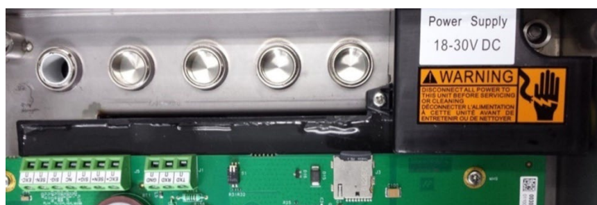
Figure 2-5: DC Power input Connector with Cover
