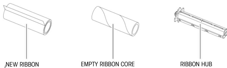
Figure 2-3: New Ribbon and Empty Ribbon Core
