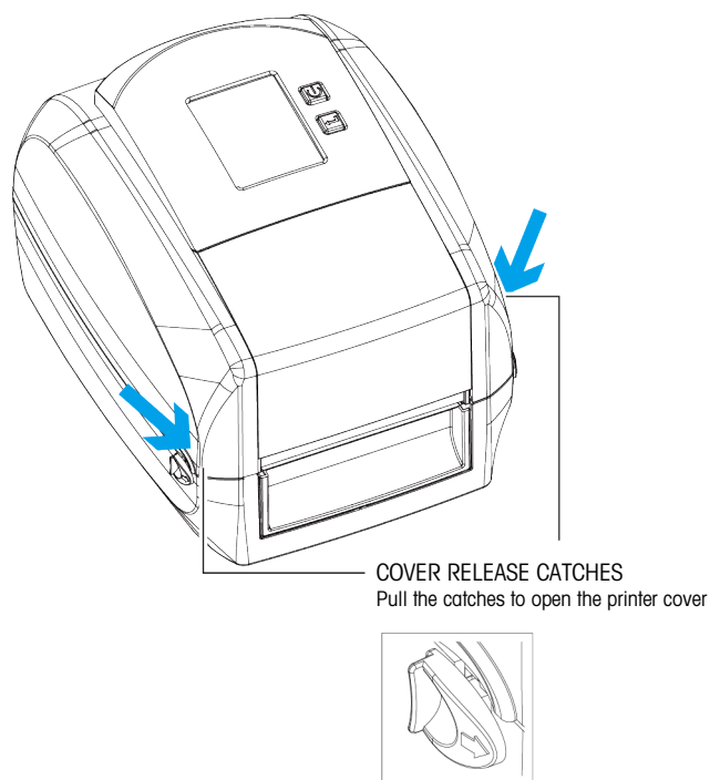
Figure 2-1: Cover Release Buttons
