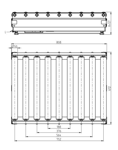
H Adjustable with 4 foot bolts Min. H = 115 mm Max. H = 140 mm
