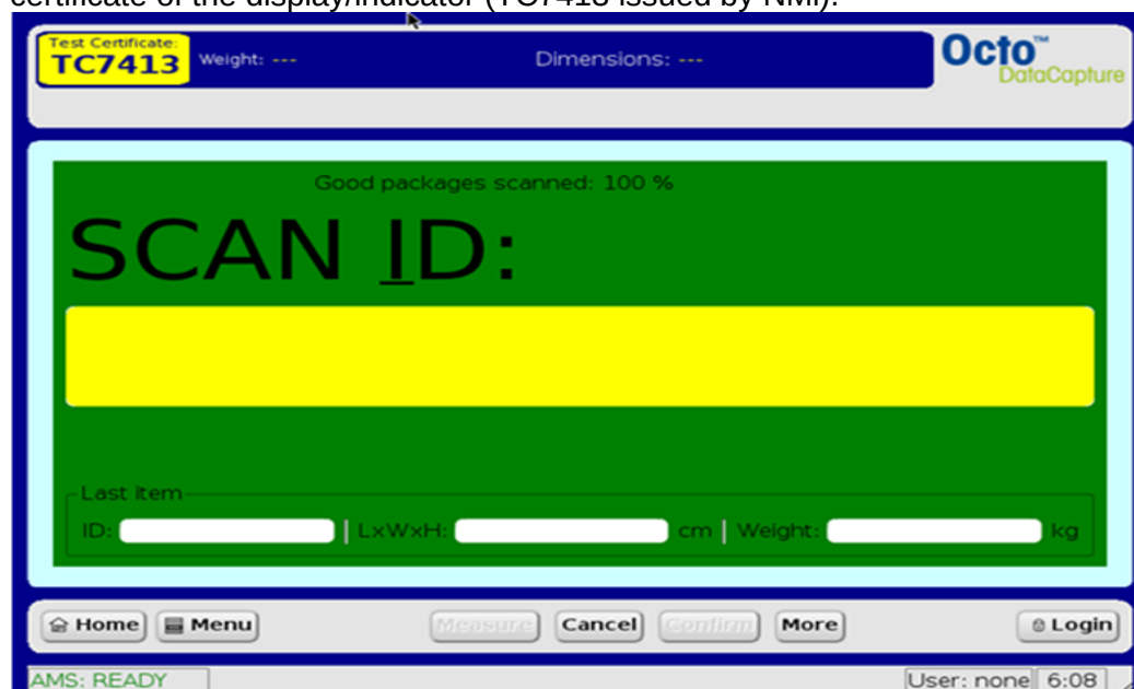
Figure 3 OctoCSM display/indicator (Upper blue field). Click on Octo logo will bring up a new page with system and seal status information.
