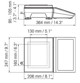
ICS4\_5 compact scale with XS weighing platform and windshield
