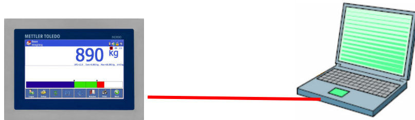
Figure B-1: Crossover Cable Connecting IND900 to a PC
