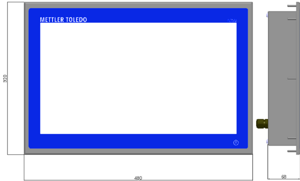
Figure 1-6: Dimensions of IND970-19, Panel Mount
