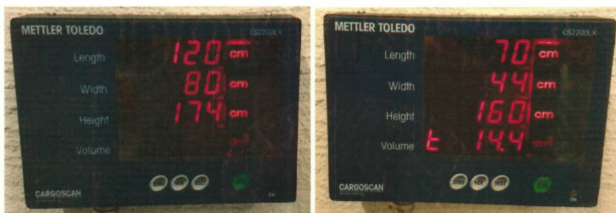
Figure 1: Cargoscan CS220 Display. Left: No Tare value. Right: Tare value=14.4cm
