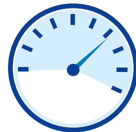
Figure 3: A tachometer only tells you how fast the engine is turning, not how fast the car is moving.
