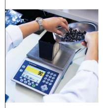
While counting pieces or checking completeness using a weighing system, operators typically have to concentrate intensely on the indicator display which slows down their process. The colorWeight<sup>®</sup> function clearly indicates, using different colors, when the target is reached. This eases the operator's concentration, speeds up the task and saves time and money.
