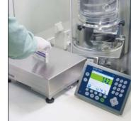
When product integrity matters, check-weighing is a fast and cost-effective quality assurance method. Whether you need to detect missing components of assemblies or whole shipments, control the completeness of castings or verify the amount of lubricants applied, the ICS scales provide clear information as to whether the quality specifications are met and the shipment is complete.
