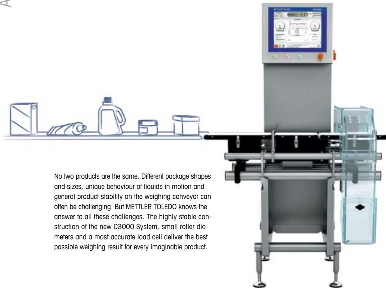
No two products are the same. Different package shapes and sizes, unique behaviour of liquids in motion and general product stability on the weighing conveyor can often be challenging. But METTLER TOLEDO knows the answer to all these challenges. The highly stable construction of the new C3000 System, small roller diameters and a most accurate load cell deliver the best possible weighing result for every imaginable product.
