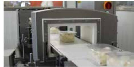
The metal detector offers optimum sensitivity to all metal types including ferrous, non-ferrous and even difficult to detect stainless steel.
