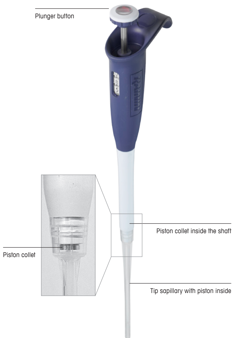
Figure 2: Positive displacement liquid end with capillary/piston attached
