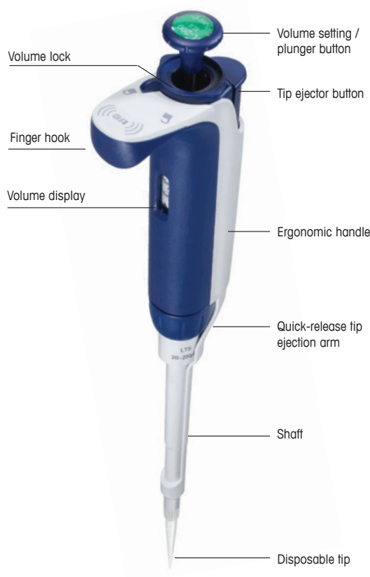
Figure 3: A manual single channel pipette.
