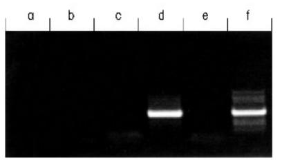
Lane (a) Tube 1 Reaction 1 = Extract from Test 1 (Cleaned pipette extract) Lane (b) Tube 2 Reaction 2 = Filter extract from Test 2 (Tip with filter) Lane (c) Tube 3 Reaction 3 = Pipette barrel and shaft extract from Test 2 (Tip with filter) Lane (d) Tube 4 Reaction 4 = Pipette barrel and shaft extract from Test 3 (Tip without filter) Lane (e) Tube 5 Reaction 5 = Negative control. Sterile water Lane (f) Tube 6 Reaction 6 = Positive control 30 pg human genomic DNA
