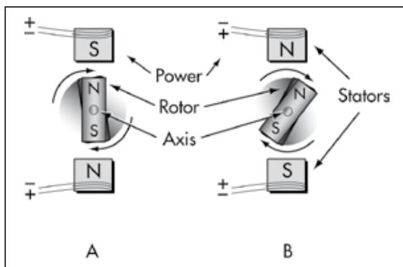
Figure 1- Stepper / motor sequence
