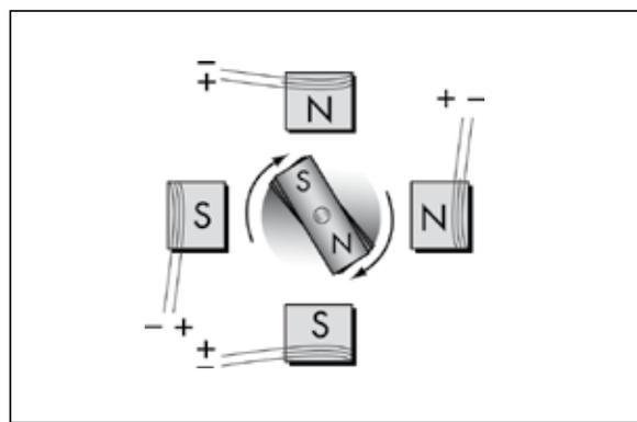
Figure 2- Multiple stators
