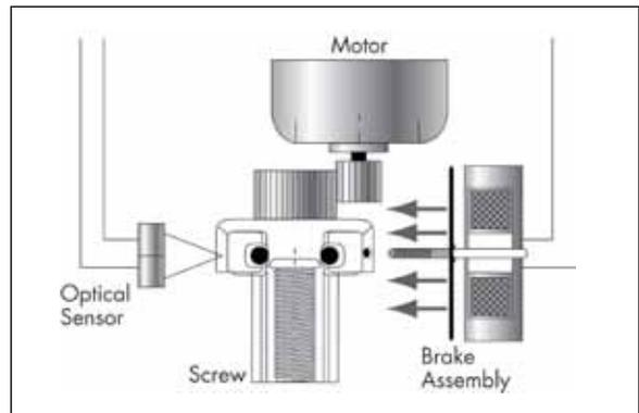
Figure 4- Mechanisms of a DC motor system
