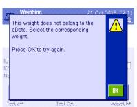
The balance firmware validates the certificate and weight data before allowing the balance test to begin. Please contact your local METTLER TOLEDO representative for more information on compatible balance firmware versions and their availability.
