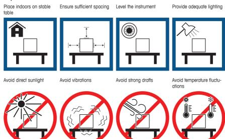
Sufficient spacing for balances: > 15 cm all around the instrument Take into account the environmental conditions. See "Technical Data."
