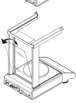
9 Remove weighing pan, pan support and bottom plate. After cleaning, reinstall all components in the reverse order. For balance mounting, refer to "Assembling the balance".
