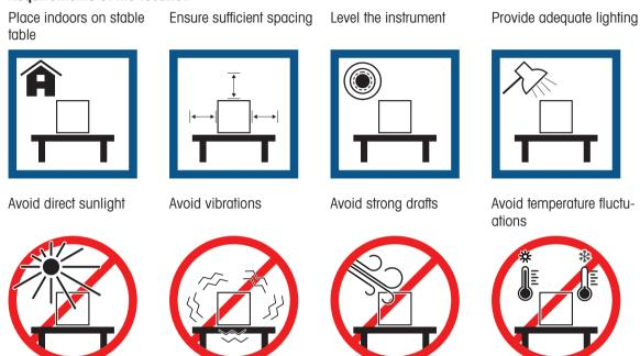
Sufficient spacing for balances: > 15 cm all around the instrument Take into account the environmental conditions. See "Technical Data".
