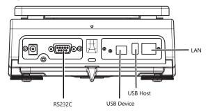
Interfaces and possible connectivity of peripheral devices:
