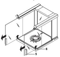
10 Push the lock button (7) to release the rear glass.
