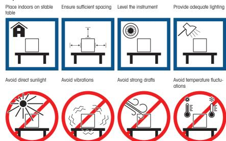
Sufficient spacing for balances: > 15 cm all around the instrument Take into account the environmental conditions. See "Technical Data".
