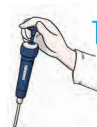
**1** First, after preparing the vessel and taring the balance, adjust the pipette to 100 percent of its nominal volume and load the manufacturer's recommended tip.
