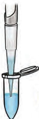
**4** Carefully move the pipette over the vessel on the balance and dispense the water. Slide the tip up the side wall to remove any excess liquid.
