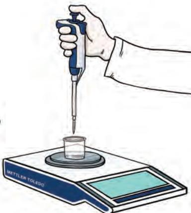
**3** Holding the pipette vertically immerse the tip to the appropriate depth and aspirate the deionized water.
