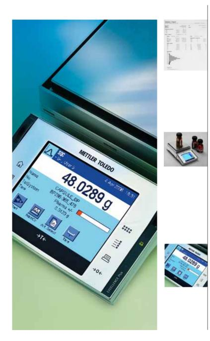
Independent standalone system SQC-XP works independently of other systems, such as networks, computers or servers. After each sample, the results are printed and statistical data is saved in the article database. As soon as a batch or a particular period of time has concluded, the statistics are printed and deleted in the system.
