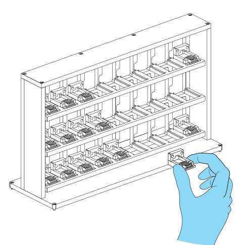
5 Place the weights on the respective weight carriers using the delivered tweezers. Do not touch the weights by hand. Pay attention to place the weights the right way on the right carrier type.
