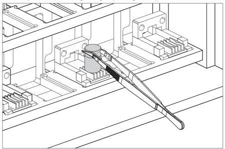
6 Once the magazine is loaded, close the weighing chamber doors.
