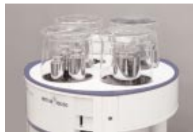
Weight handler for automatic mass determination with single weight or group of weights
