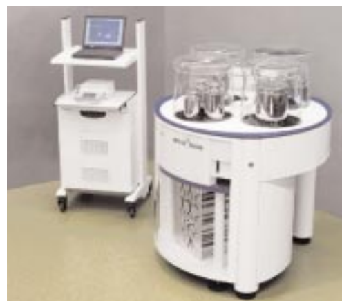
Individual draft shield for stable environmental conditions
