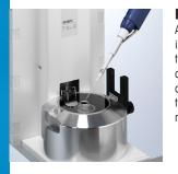
Fast and Ergonomic As soon as a pipette passes through the integrated light barrier, the evaporation trap opens automatically. Technicians can concentrate on the calibration process without worrying about operating the balance. Suitable for both left and right handed users.
