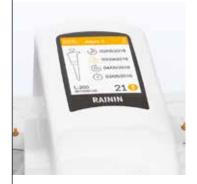
SmartStand displays the check, calibration and service dates that can be stored on every Rainin XLS pipette.
