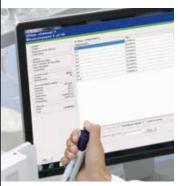
Sophisticated calibration software for full customer traceability of calibration data, which is stored in a secure database for ISO 8655 and allows regulation complaint reports.
