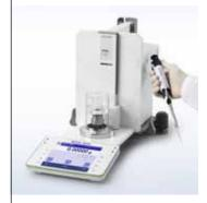
With an RFID tagged pipette, the check is automatically initiated. The tag contains the pipette data, check interval and method. When a check is passed the next date is stored on the pipette.
