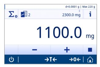
The **Totaling** application allows the user to weigh different samples, add their weight values and totalize them. The application allows the user to:
